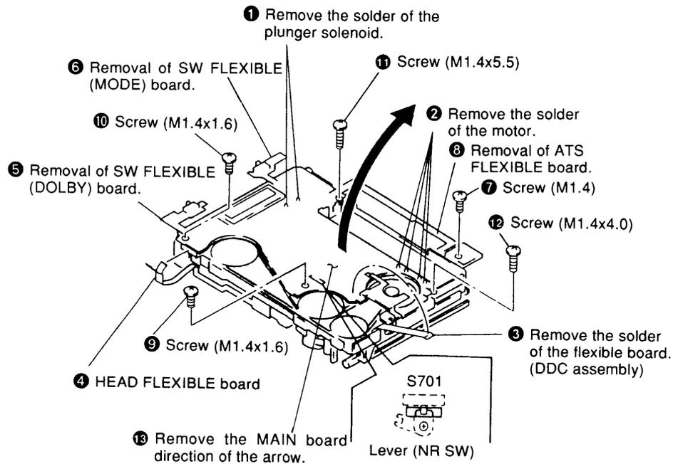
Note : Confirm if the switch lever installs itself in the groove of a lever (NR SW) for assembling.
