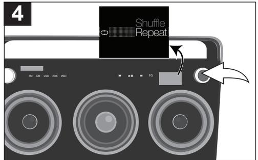
Press the OK button once more; the Repeat All indicator ② will light and all songs in the selected folder will repeat continuously. Press the OK button to confirm the setting or wait a few seconds to go back to the previous menu.
