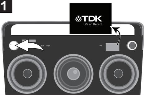
Turn this unit on by rotating the Volume/Power control until a click is heard and the Power indicator lights to turn the unit on.
