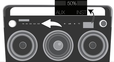
Press the INST (Instrument) button/indicator to select Instrument; the MIX menu will appear in the Main display.
