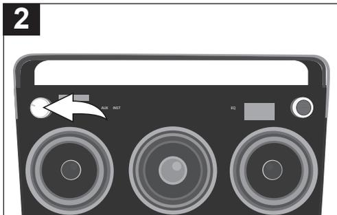
2 Rotate the Volume/Power control clockwise to increase or counter-clockwise to decrease the volume.
