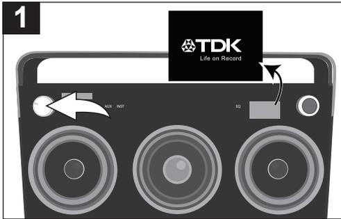
Turn this unit on by rotating the Volume/Power control until a click is heard and the Power indicator lights to turn the unit on.
