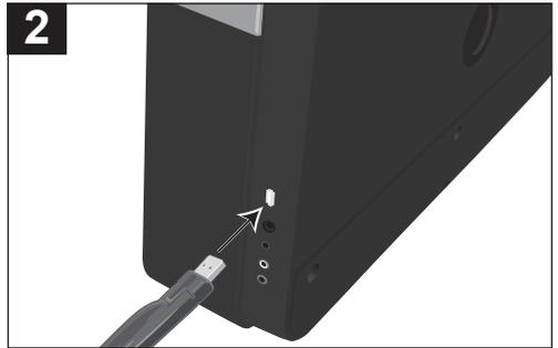
Insert a USB drive (support up to 32GB) into the USB jack. This unit supports MP3/WMA with a Bit Rate up to 320kbps.
