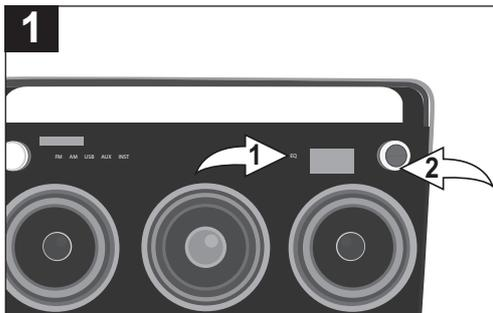
1 During any mode, press the EQ button/indicator ❶; *Bass* will appear in the Main display. Adjust the Bass as desired using the Select control ❷.
