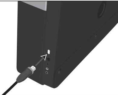
Insert the iPod cable to the iPod and the other end with the USB plug into the USB jack on the side of this unit.
