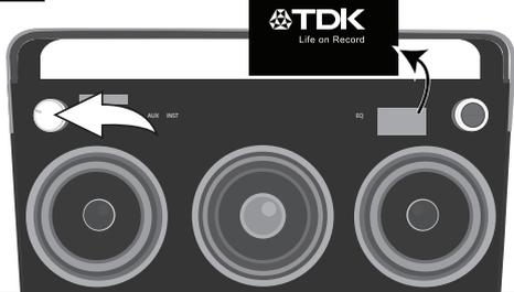
Turn this unit on by rotating the Volume/Power control until a click is heard and the Power indicator lights to turn the unit on.
