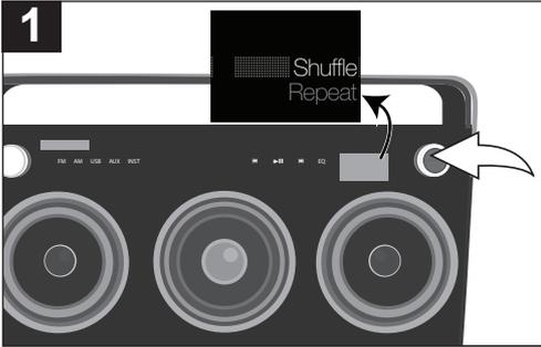
While in the Play or Paused USB mode and with a USB device inserted, press the OK button; *Shuffle* and *Repeat* will appear in the Main display.
