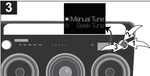
While the frequency appears in the display, press the OK button ❶; *Manual Tune/Seek Tune* will appear in the main display. Using the Select control ❷, select *Manual Tune* to adjust the frequency one step at a time, or *Seek Tune* to have the unit automatically go to the next strong station; then press the OK button ❶. Press the BACK button ❸ or wait a few seconds to return to the station view.
