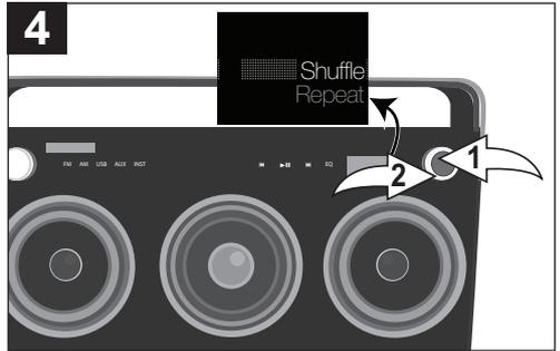
To cancel Random playback, press the OK button ① to bring up the Shuffle/Repeat menu. Select Shuffle using the Select control ②, and then press the OK button ① again;  $\times$  will disappear. Press the OK button ① to confirm the setting or wait a few seconds to go back to the previous menu.
