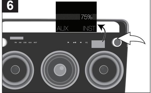
Select the desired ratio using the Select control. For example, to make the Instrument more dominant, rotate the Select control clockwise to increase the Instrument ratio.
