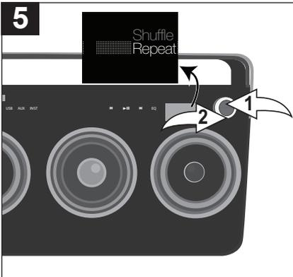
To cancel Repeat playback, press the OK button ① to bring up the Shuffle/ Repeat menu. Select Repeat using the Select control ②, and then press the OK button ① repeatedly until the Repeat indicators disappear.
