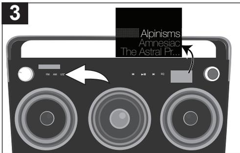
Press the USB button/indicator to select USB; the list of folders/files will appear in the Main display.
