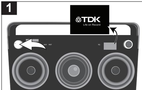
1 Rotate the Volume/Power control until a click is heard and the Power indicator lights to turn the unit on.
