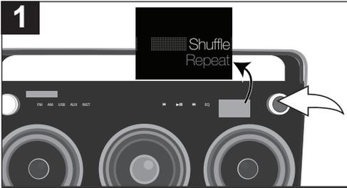
While in the Play or Pause USB mode and with a USB device inserted, press the OK button; *Shuffle* and *Repeat* will appear in the Main display.
