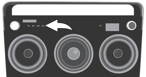
Press the AUX button/indicator once to select the AUX1 mode (LINE IN jack) or twice to select the AUX2 mode (RCA IN jack) and start playback of the external device.
