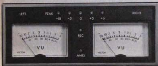
Five LED peak level indicators eliminate under-recording and tape saturation.
