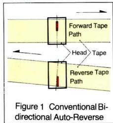
As long as the tape moves in one direction, equilibrium is established. The tape carries the guide to one side and it stays there. But when direction is reversed, the tape
