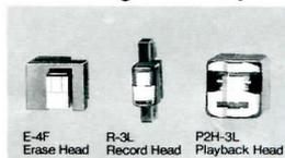
The CR-3 uses physically independent ("discrete") record and play heads that are magnetically aligned *after* installation to ensure flat response, maximum headroom and minimum noise. The heads are individually shielded to prevent crossfeed and
