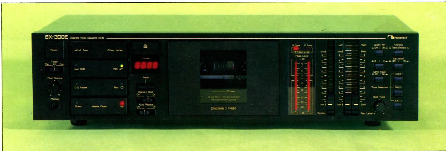
Of the Nakamichi range, the BX-300E is in my view the top domestic recorder. Above lie machines with professional facilities but little extra performance. Inevitably, it uses a dual-capstan transport for speed stability, with direct drive to the main capstan. A unique pitch control changes speed by around +/-6%.
