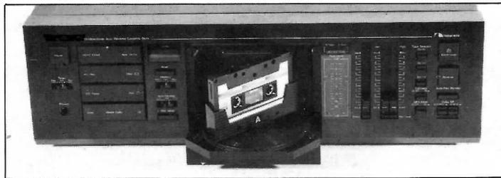
As Nakamichi's top auto-reverse deck, this model is pretty expensive. Its main claim to fame - and incredulity - is the way auto-reverse is implemented. To avoid problems associated with rotating the head, Nakamichi instead rotate the cassette. It flies out of the machine on a tray, spins round like a ballerina then whizzes back in again. This performance leaves no one unmoved!
