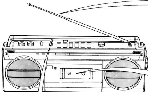
When lifting the unit by the handle, the telescopic rod aerial should not be raised because it may be bent or torn off.
