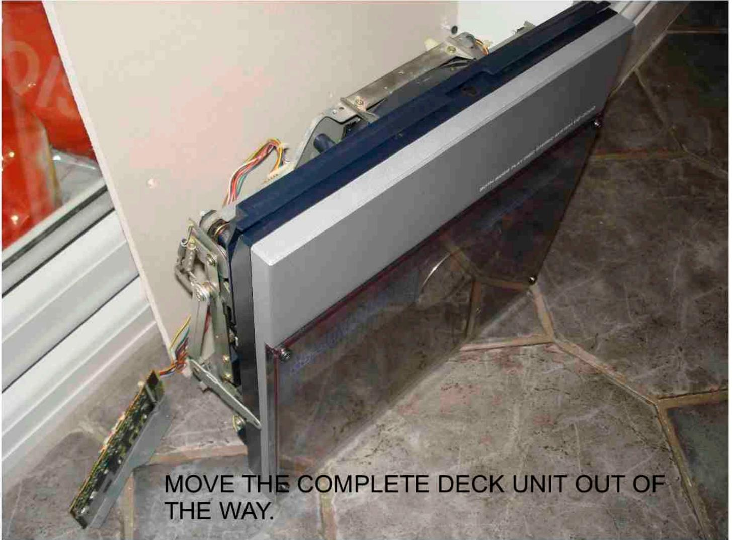
MOVE THE COMPLETE DECK UNIT OUT OF THE WAY.
