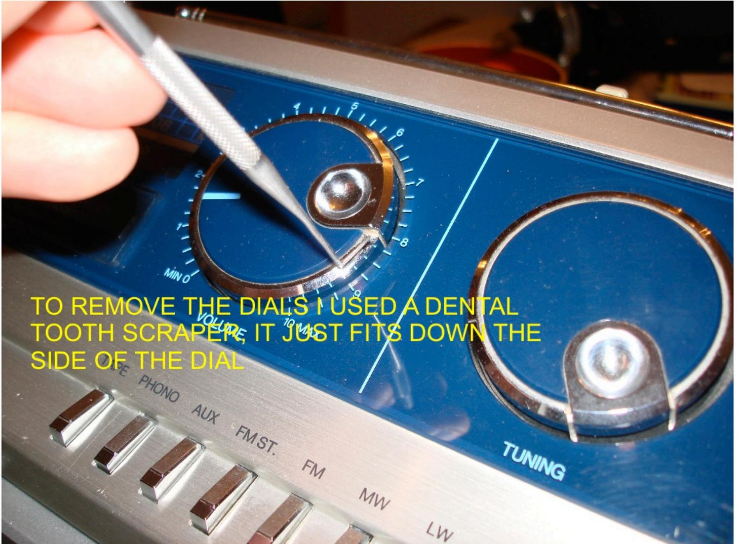
TO REMOVE THE DIALS I USED A DENTAL TOOTH SCRAPER, IT JUST FITS DOWN THE SIDE OF THE DIAL
