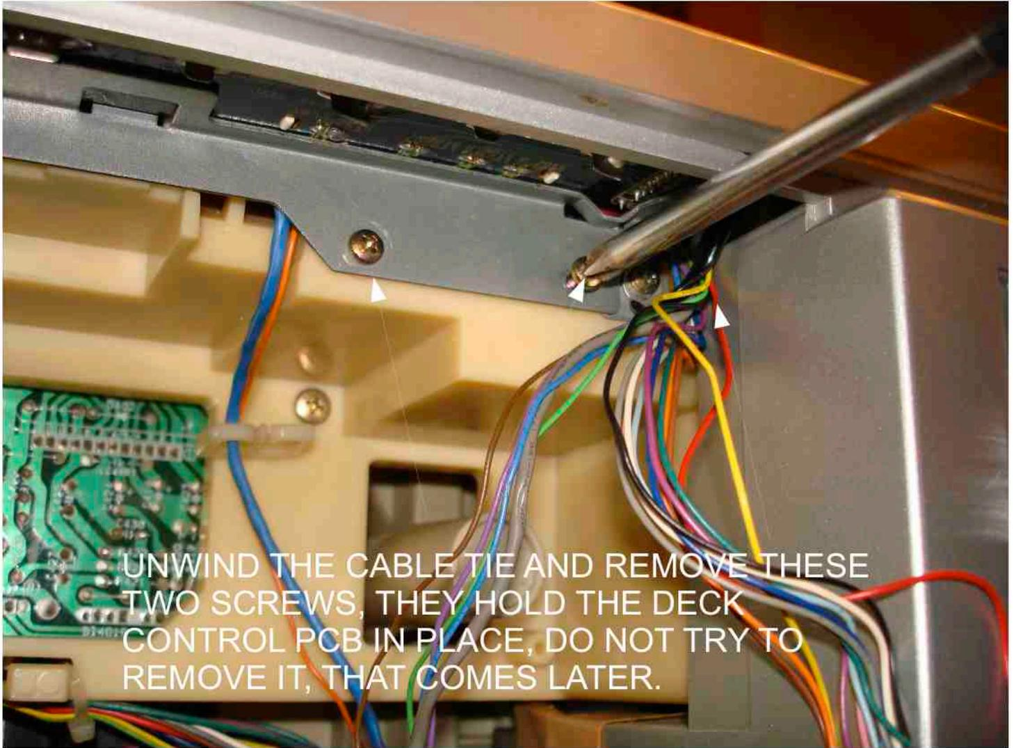
UNWIND THE CABLE TIE AND REMOVE THESE TWO SCREWS, THEY HOLD THE DECK CONTROL PCB IN PLACE, DO NOT TRY TO REMOVE IT, THAT COMES LATER.
