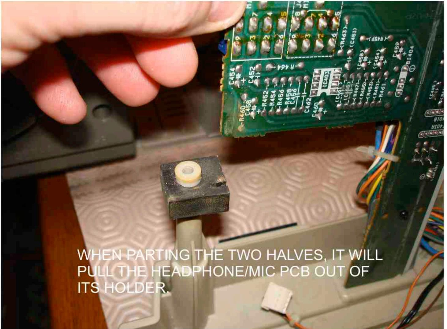
WHEN PARTING THE TWO HALVES, IT WILL PULL THE HEADPHONE/MIC PCB OUT OF ITS HOLDER.
