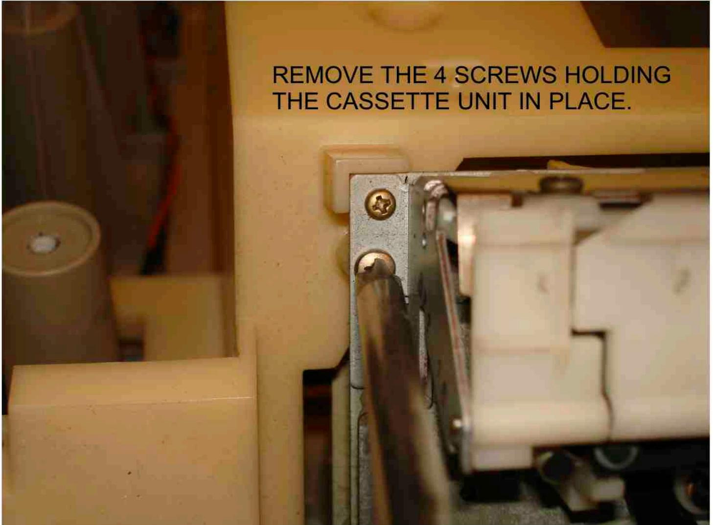
YOU WILL HAVE TO TWIST AND FIDDLE ABOUT TO GET THE UNIT OUT OF IT MOUNTING, WHEN YOU DO REMOVE THIS FROM THE CASSETTE UNIT, REMEMBER HOW IT FITS BACK ON, ITS A PAIN TO GET BACK ON AS WELL. I USED A PAIR OF NARROW NOSED PLIARS.
