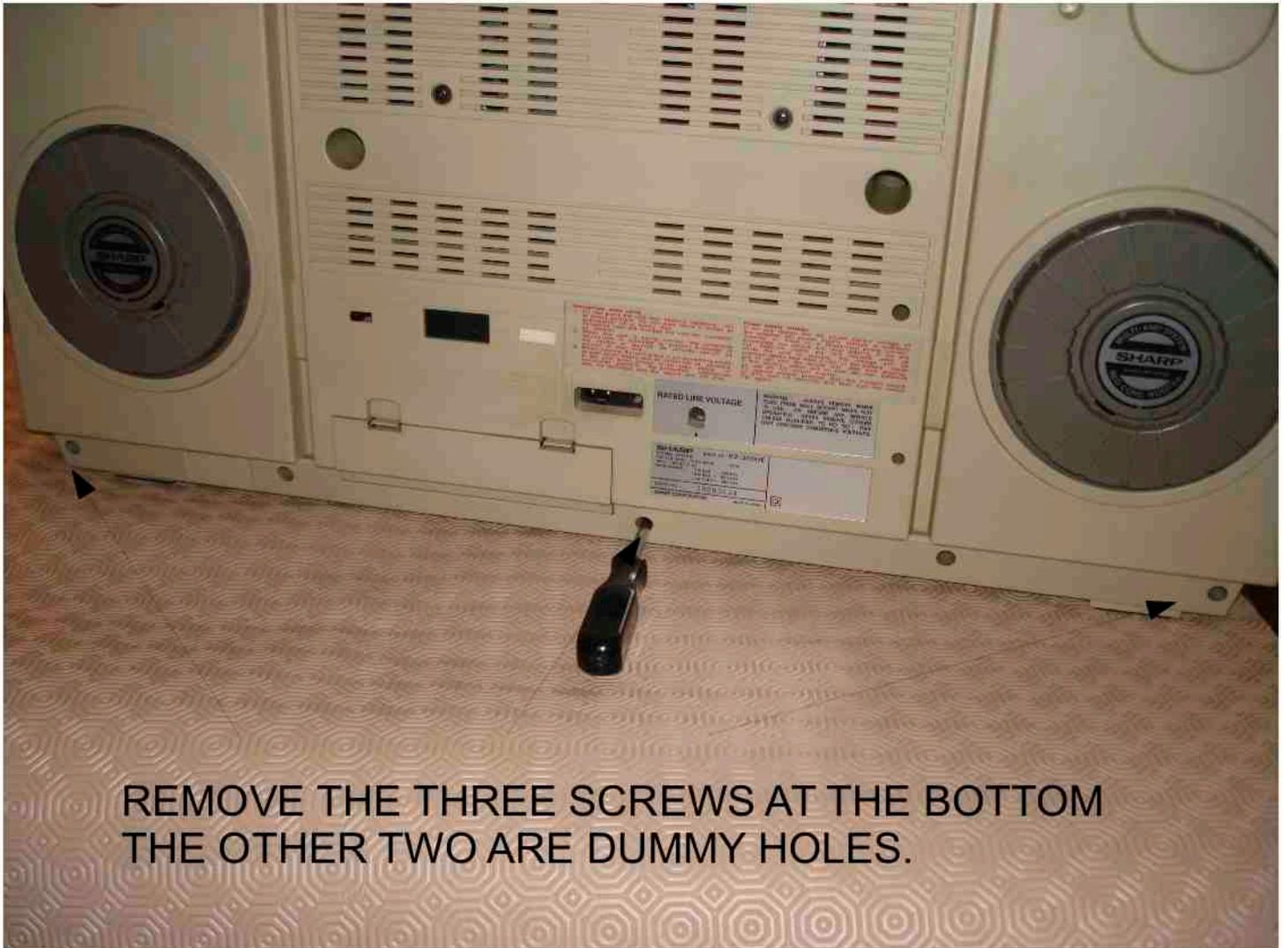
REMOVE THE THREE SCREWS AT THE BOTTOM
