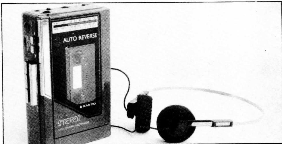
The MG-95 is an auto-reverse unit with a built in FM/AM radio that has stereo on FM. Optional reverse modes weren't available; it keeps on reversing at both ends of a tape until manually stopped. Dolby is not fitted.
