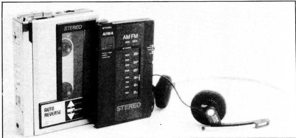
This little unit felt and looked better made than most. Its metal case was sturdy, well finished and particularly smart. The construction didn't introduce any weight penalty though; the HS-U07 weighed a low 230gms and had compact dimensions too.
