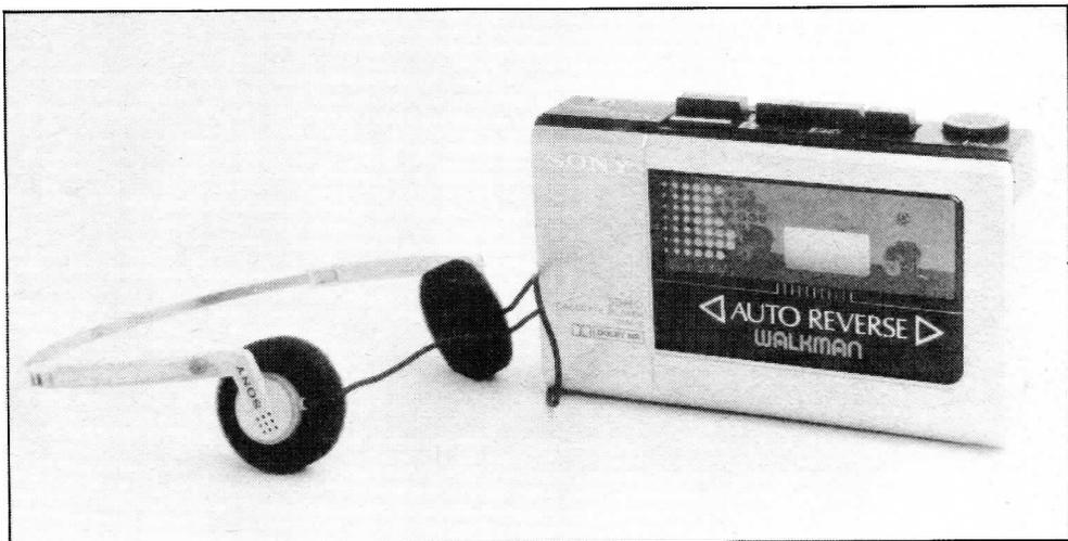
This is an auto-reversing player fitted with Dolby noise reduction. As Sony's Walkmans go, it is large; it is also made of plastic and both felt and looked inferior to Sony's original metal Walkmans. A shoulder strap is supplied with this unit, but not a pouch.
