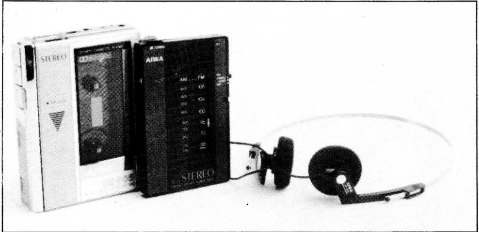
The HS-P06 is distinguished by its small size and light weight. Although well made and fairly solid in feel, this personal stereo weighs just under 200gms — lighter than most. As usual though, small size means small batteries (two AAA's) and limited battery life.
