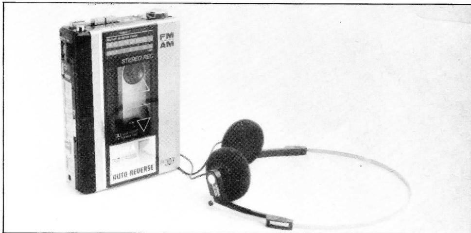
This unit has a built-in radio, unlike the HS-U07 where it comes as a cassette insert. Built in radio is more convenient and has the benefit that recordings can be made from it. Aiwa have fitted the J07 with record circuitry, allowing it to record from radio, a microphone or a line source. Dolby noise reduction has also been fitted, but it only acts on cassette replay.
