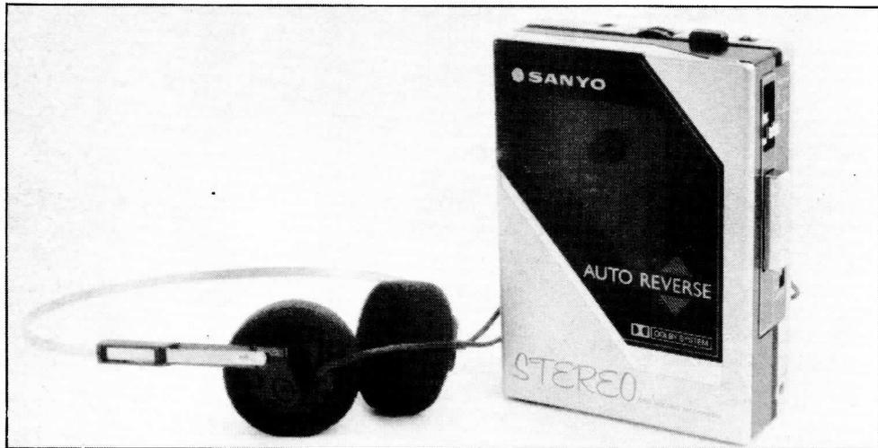
The MG-80D is a light and compact player, lacking radio but fitted with Dolby B noise reduction. As a result, it plays Dolby cassettes properly, avoiding the hissy brightness that non-Dolby machines suffer with such recordings.
