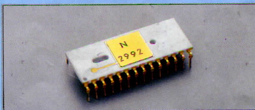
16 BIT D/A Converter
