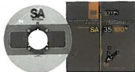
This tape brings the benefits of an advanced cassette tape formulation to open-reel recorders. It offers dramatic improvement in quality, especially at lower speeds, on those machines fitted with a suitable EE bias setting. This is equivalent to the High Bias/35 µs equalisation setting. This tape is not available with back treatment.
